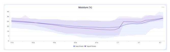
This example comparing two Scout Groups (Deep Scouts & Topsoil Scouts) shows that 1.7. rain has quickly wetted the topsoil and diminished variability, while deep soil reacted several days later and less dramatically.
