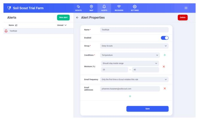
In this example the rule "TestRule" will start monitoring that Scouts in the "Deep Scouts" group stay inside the desired moisture range 25-40 %. If a measurement value outside the range is received, the email recipent will get notified. When a second group member triggers the condition, a new email will not be sent.
