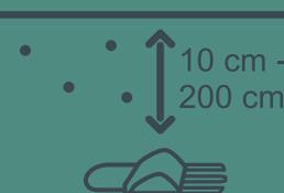
Soil Scout sensors can be placed at multiple depths. The patented underground wireless technology is tested for 2 meters (6 feet) below the ground.
